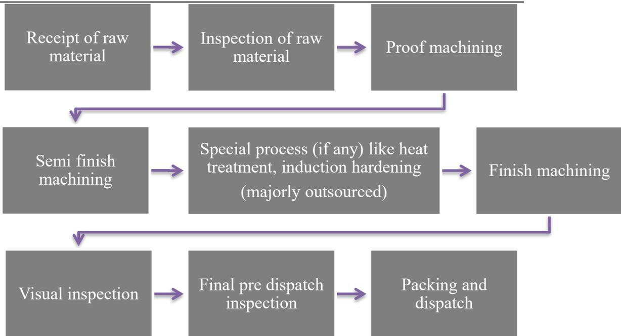
The process undergone in the manufacturing of precision machined components is briefly described hereunder:
